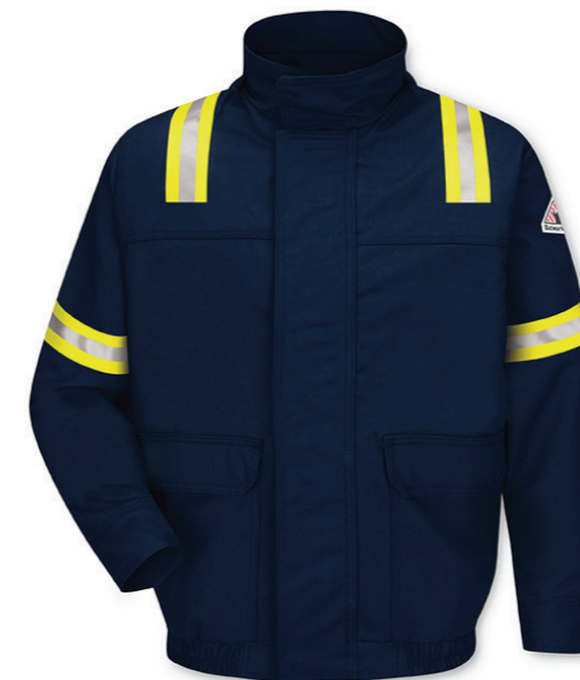
9585 E-VIS EXCEL FR® BOMBER JACKET 88% Cotton/12% high tenacity Nylon with 7oz. 100% cotton lining Navy (20) ATPV 30.4 | ARC 3 | UL 2112 Certified Does not meet ANSI 107 visibility requirement for Hi-Vis garments.
